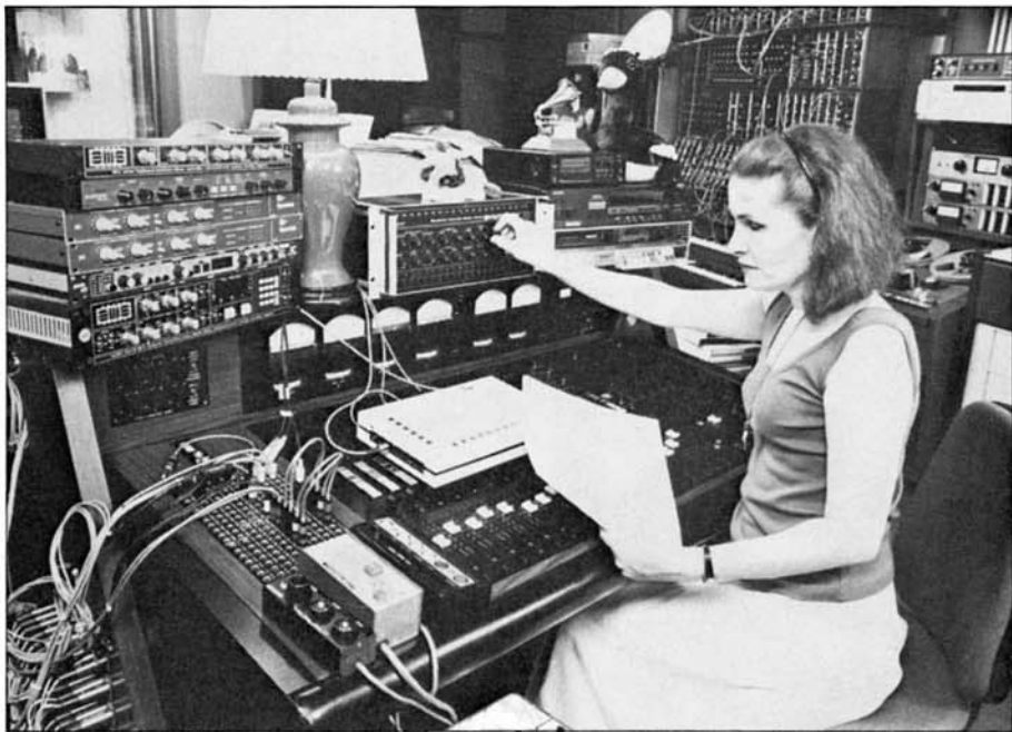
Carlos at her custom-built mixing desk, on which rests (L, top to bottom) AMS keyboard control module, Synton 216 vocoder, two Symetrix 511 noise reduction units, Lexicon PCM 42 DDL, AMS dmx 15-80S pitch shifter/DDL; (center) Synton 221 vocoder; (R) Nakamichi DPM-100 2-track digital recorder on top of Sony PCM 701 and Betamax VCR. Moog modular system, 2-track vocoder, and Moog string filter stand in background to right. Fairlight Voicetracker rests on top of mixing desk.
