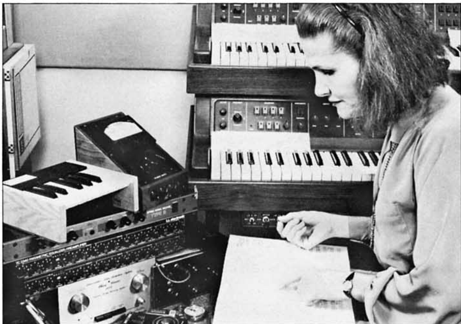
Wendy with some of the tools of her trade (L, top to bottom): one-octave keyboard used to remotely control Hewlett-Packard computer, volume and tone controls, Aphex Aural Exciter Type B, T.C. Electronics parametric equalizers, Phase Linear Autocorrelator, Moog 904 lowpass filter. Two Synergy synthesizers stand to the rear. Note custom switch used to control which Synergy is affected by Hewlett-Packard tuning tables.
